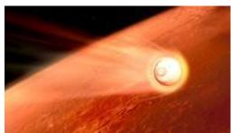
**Perseverance Rover Decelerating in the Martian Atmosphere (Illustration)**: In this illustration of its descent to Mars, the spacecraft containing NASA's Perseverance rover slows down using the drag generated by its motion in the Martian atmosphere. Credit: NASA/JPL-Caltech. <u>Full image and caption ></u>
